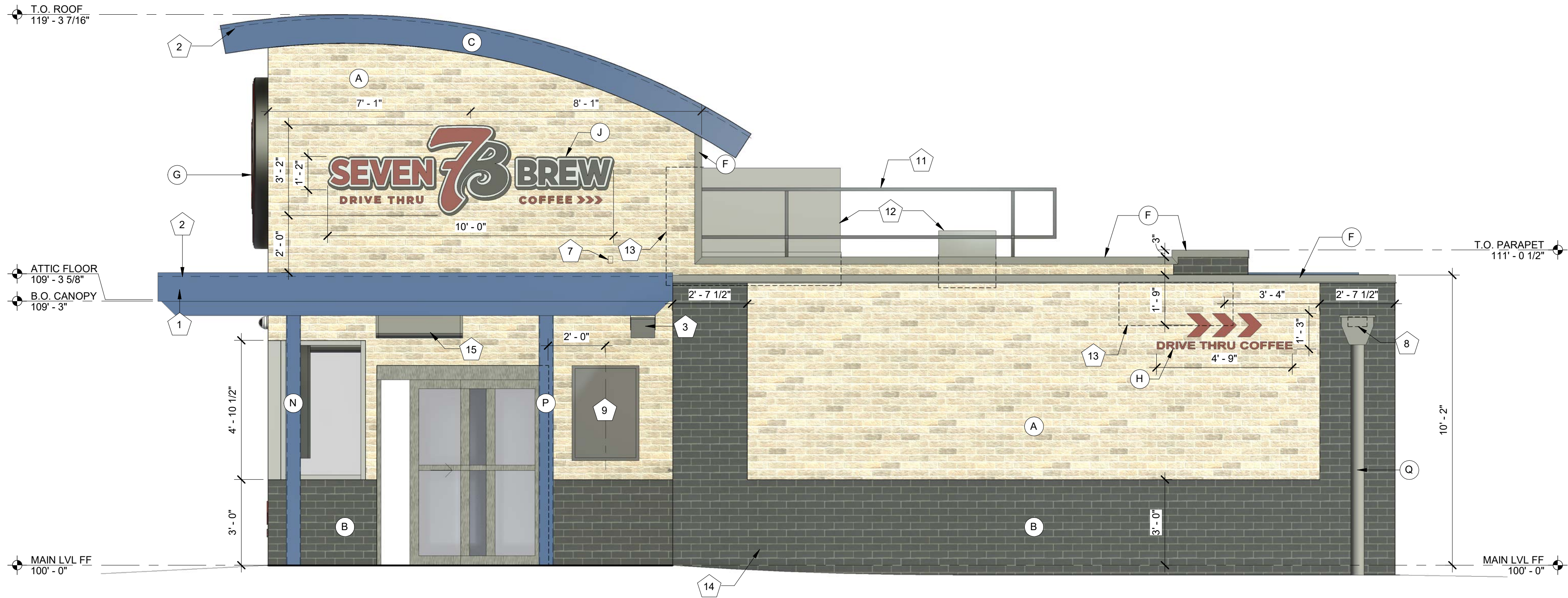
2 EXTERIOR ELEVATION - LEFT W/ COOLER 3/8" = 1'-0"
