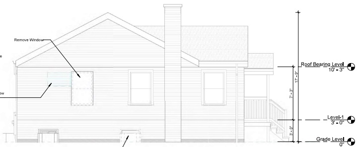
① Existing South Elevation 1/4" = 1'-0"
