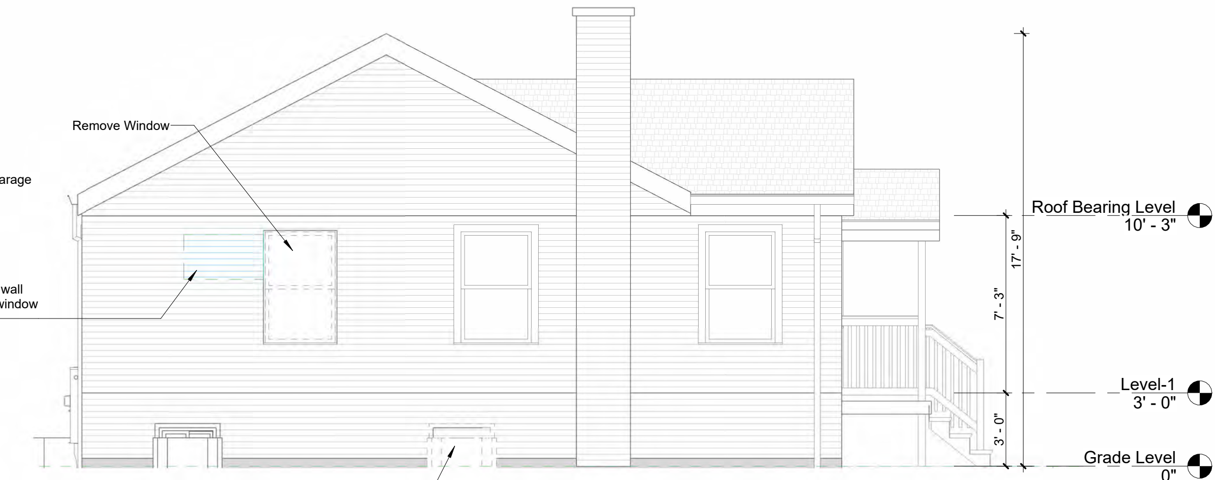
① Existing South Elevation 1/4" = 1'-0"
