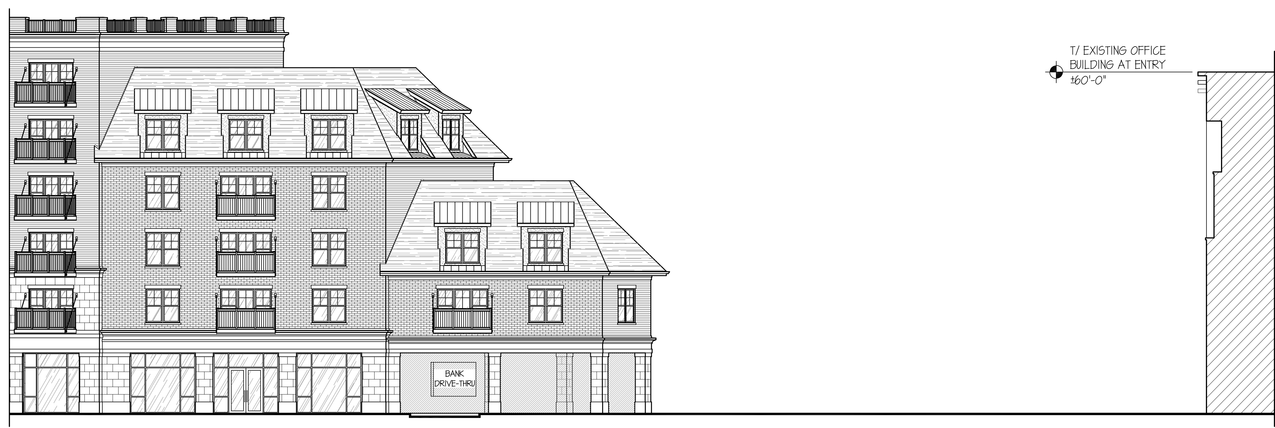
PROPOSED EAST (PARKING LOT) ELEVATION SHOWN W/ EXISTING ADJACENT OFFICE BUILDING REFERENCE
