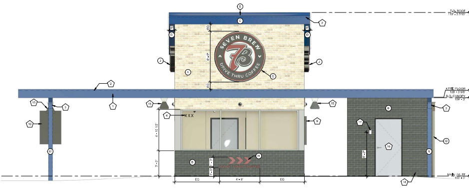
1 EXTERIOR ELEVATION - FRONT 3/8" = 1'-0"
